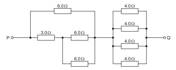
What is the resistance between the points P and Q due to the resistance network?
