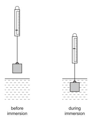
A reduction in the balance reading occurs as a consequence of the immersion.
